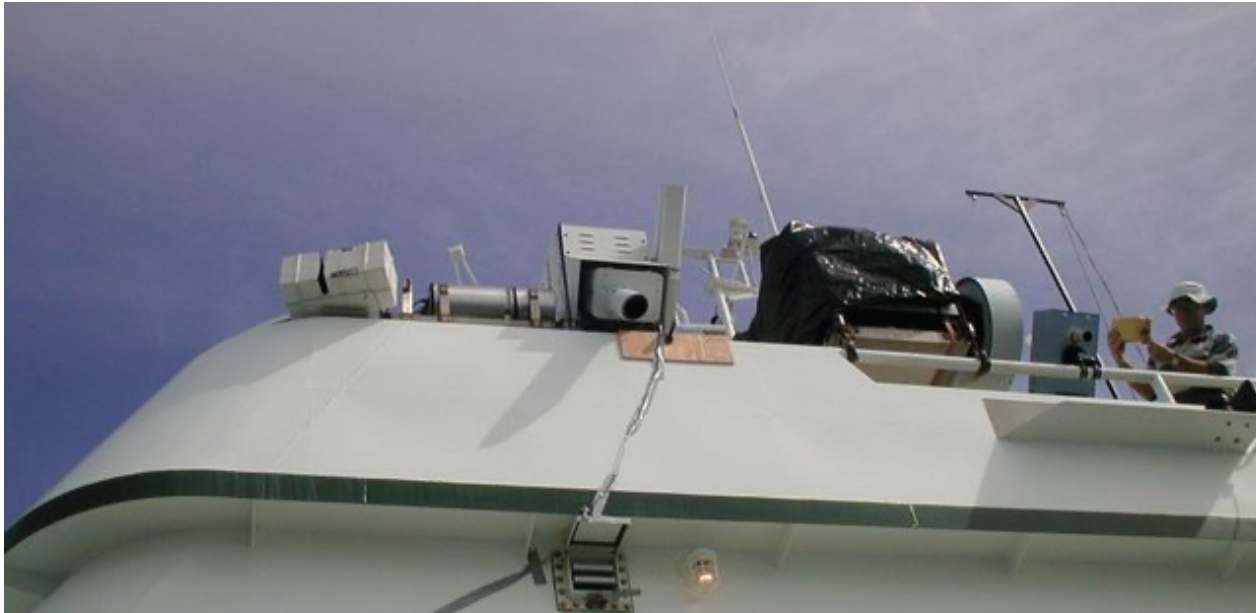
From left to right: SISTeR, ISAR, CIRIMS, M-AERI and DAR011 on the R/V F.G. Walton Smith in 2001
